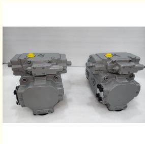
Fig. 2: Assembly of the A4VSO series 1, 2 and 3
